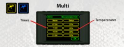
Multi mode allows 4 different periods of temperature control in the 24hour cycle. This allows you to create and even more realistic climate than the day and night mode. For example you can set different temperatures for Morning, Midday, Evening and Night. Not all periods have to be used. To delete a period select a period and delete the time.
